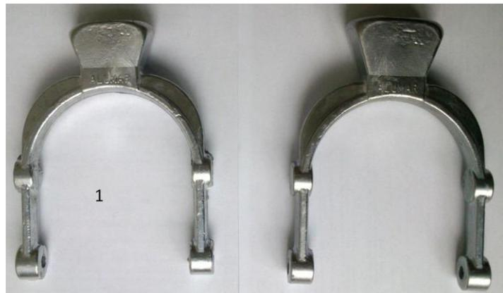
Figure 24. First casting in preheated mould on 200 °C and casting from a mould with stabilised temperature field (higher mould temperature)
