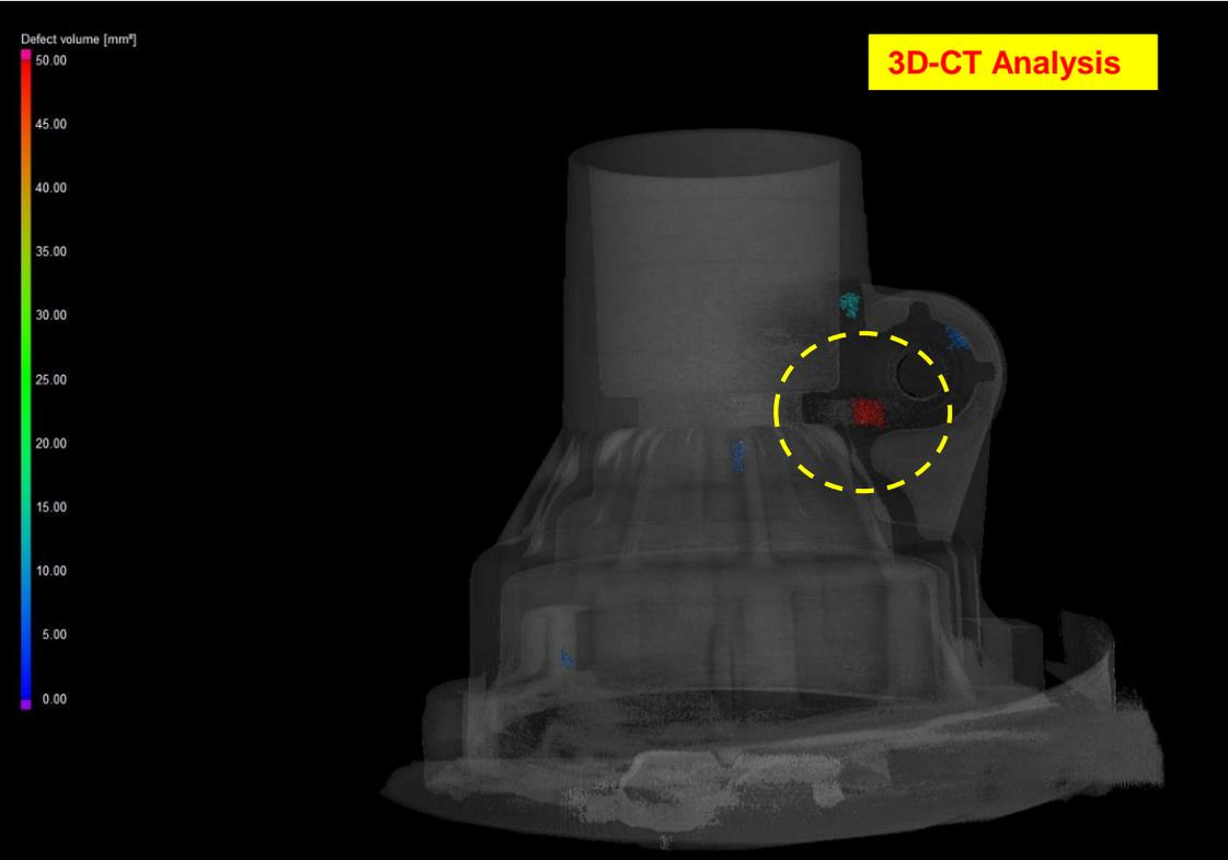
\*Presented shrinkage porosity areas are not allowed, with help of the local squeezing can be eliminate
