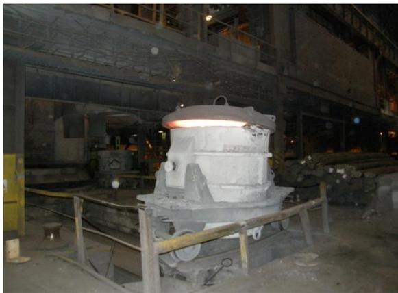
Figure 1. Ladle and its cover with a thermal insulation layer
