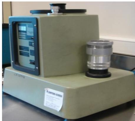
Figure 4. Permeability tester with accessory attached
