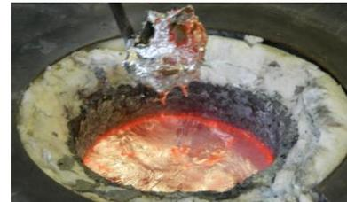
Figure 5. Removing slag from the melt
