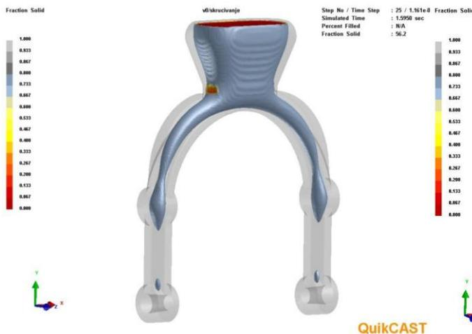
Figure 19. Fraction solid result after 1.6 seconds in radiographic view
