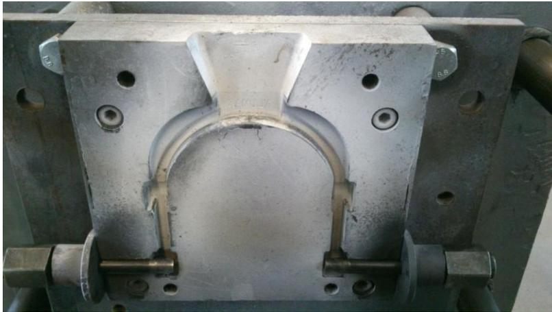
Figure 6. Coated mould surface before casting cycles
