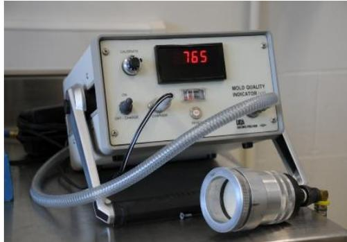
Figure 5. MQI with accessory attached
