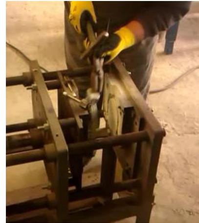
Figure 7. Removing casting out from the mould
