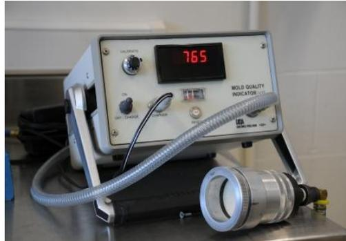
Figure 5. MQI with accessory attached
