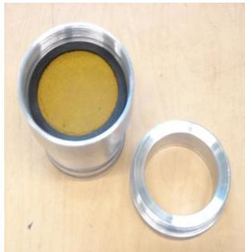
Figure 6. Specimen in gasket within holder accessory
