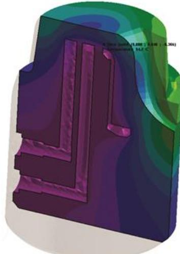
Temperature in critical area was in ver. 1- 235,3 °C, with new cooling system the temperature was 94,7 °C
