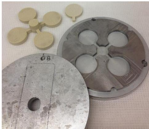
Figure 1. Four-cavity disc core box
