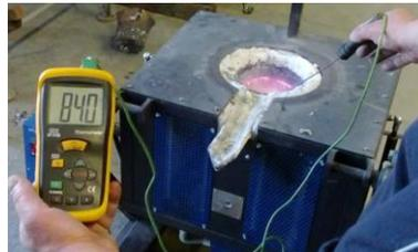
Figure 4. Measuring melt temperature
