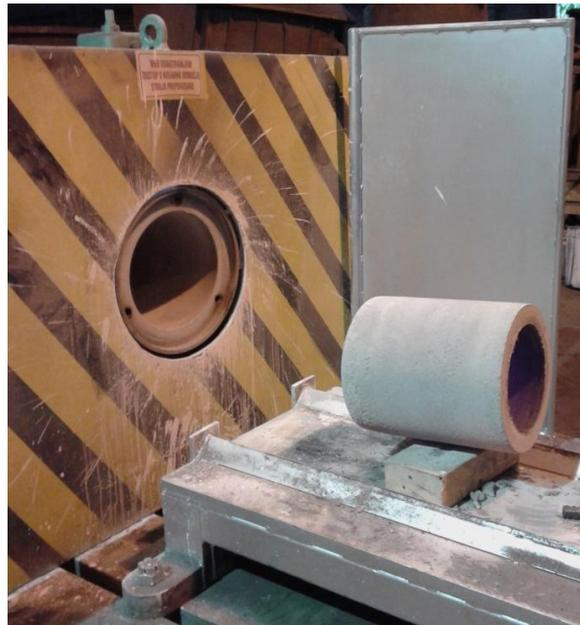
Figure 1. High carbon high speed steel hollow cylinder casting in front of the laboratory centrifugal casting device
