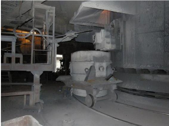
Figure 1. Ladle placed under the furnace tapping hole
