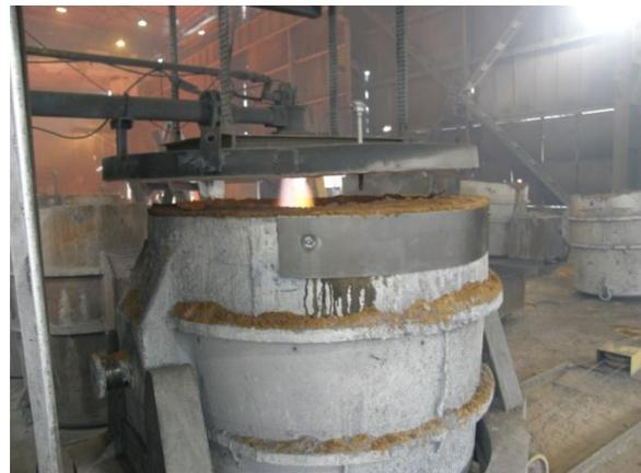
Figure 4. Unit intended for drying and soaking of casting ladles
