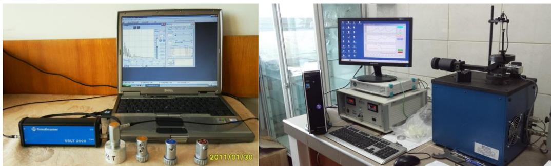
Figure 3. The damping Krautkramer USLT 2000 (left) and wear T-01 M (right) instruments used during the experiments
