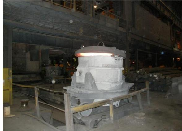
Figure 2. Ladle and its lid with a thermal insulation layer
