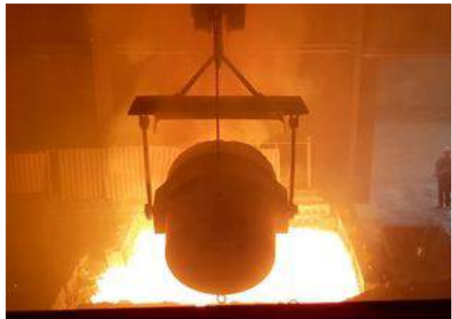
Figure 2. The process of alloy casting into a foundry box
